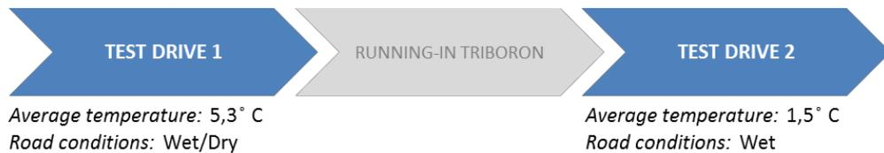
All five test vehicles were driven in a trailing row and changed places on a regular basis, i.e. all vehicles have been in all places.
