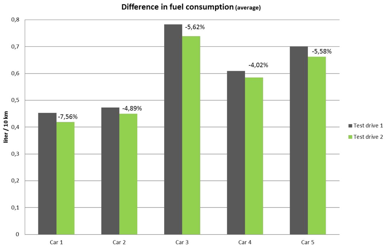
The reduction in fuel consumption was on average a bit larger for the diesel cars:
